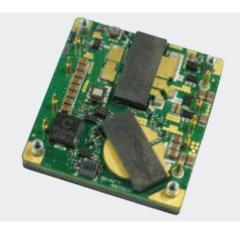
Advanced Energy's Artesyn AVE600 series half-brick isolated DC-DC converter provides a single regulated low noise 12 Vdc output that can deliver up to 50 amps. It has a wide 2:1 input range of 36 to 75 Vdc and is designed primarily for use with standard 48 V telecommunications equipment supplies. This converter is normally used in designs with a distributed power architecture (DPA), where one or more downstream non-isolated DC-DC converters meet the needs of lower voltage semiconductor devices.
