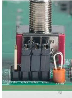
Fig. 9 – The enable jumpers – all 3 shown in place to enable all 3 outputs
