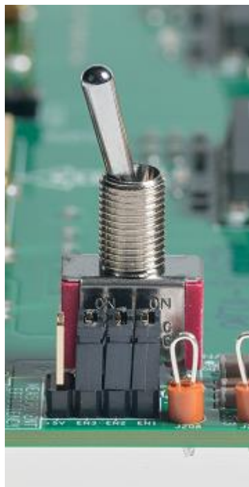
Fig. 4 – Enable jumper location and population
