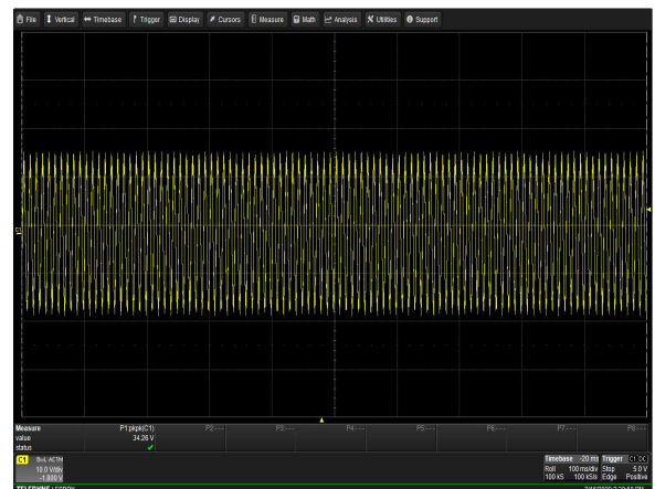
Figure 10: AIF04ZPFC-01L Ripple and Noise Measurement Vin = 230Vac Load: Io = 4.2A Co = 470uF Ch 1: Vo
