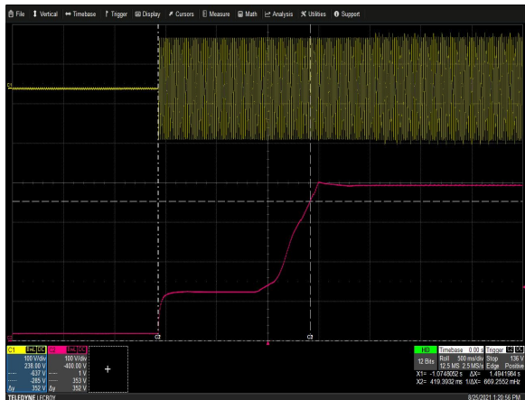
Figure 1: AIF04ZPFC-01L Turn-on delay via AC mains Vin = 90Vac Load: Io = 0A Co = 470uF Ch 1: Vin Ch 2: Vo
