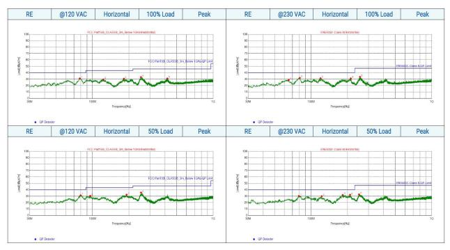
Note - Conducted and radiated emissions plots show measurements with resistive loads according to the IEC/EN/UL standard's requirements. EMC performance can be impacted by system level design, integration, or associated connections with additional wires and/or devices.
