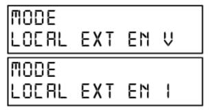
These modes allow local control of the supply in addition to using an analog input for enable/disable. You may choose to use the analog voltage input or the analog current input to be used as an external enable/disable for the power supply. Each input has an internal pull-up so you may use an external contact or a voltage signal (0-5VDC) for this function. With either input, the following functionality will be available when the mode is turned on.
