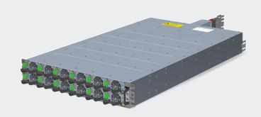
Advanced Energy's Artesyn introduces the 30 kW stand-alone Power Shelf, single voltage 48 VDC output, powered from three-phase AC line. The Power Shelf sits in a 2RU high slot in a EIA 19" rack, which hosts twelve power modules with the outputs connected in parallel. Each module is an AC/DC power converter rated at 3000 W, 48 VDC of nominal output power, hot-swappable, accurate current sharing and is self-cooled. The shelf will power the IT system through the OCP compatible busbar.
